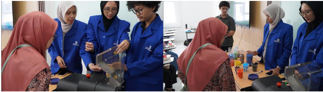
Figure 2. Bottle caps being chrushed with mechanical shredder
